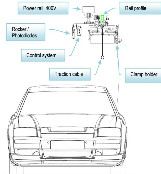
The device's photodiodes are mounted on a mobile rocker that a control system servo motor moves into a position that is calibrated to that of the vehicle panel.
