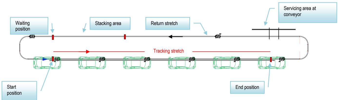
When the MBO reaches its starting position, it moves the rocker containing the photodiodes into a precalibrated position and waits until the reflected light from a vehicle panel is detected by the diodes. It then begins tracking the vehicle via the panel, keeping a constant distance from it, thus enabling the MBO to adjust its speed automatically to that of the production line.
